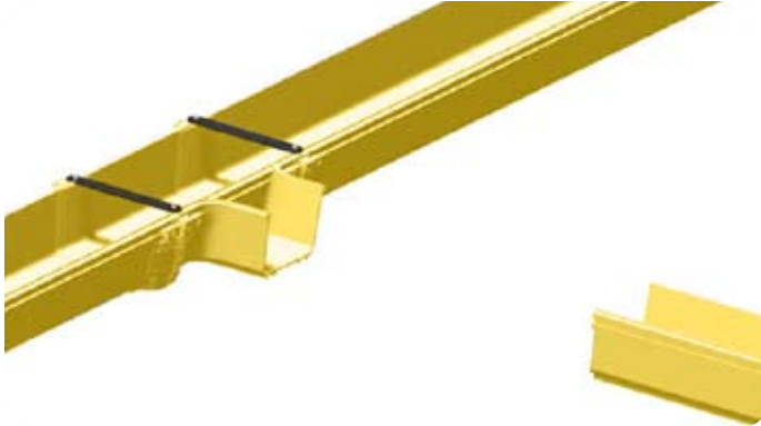
Raceway system with gap between opposing runs
